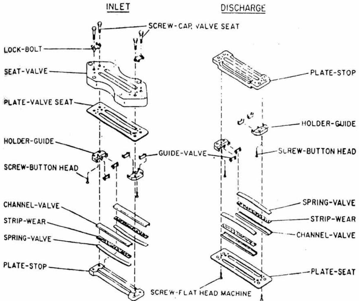
Fig. 7RN-2—Typical Type "A" NL Rectangular Inlet and Discharge Channel Valve.
